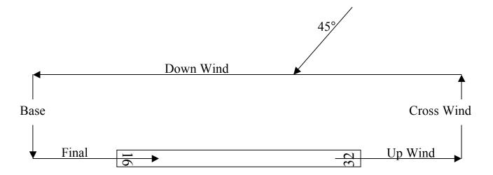
By default, turns are done to the left in what is called "left traffic". Shown above is the left traffic pattern for runway 16. Some runways are designated as having a "right traffic" pattern, which means turns to the right.
